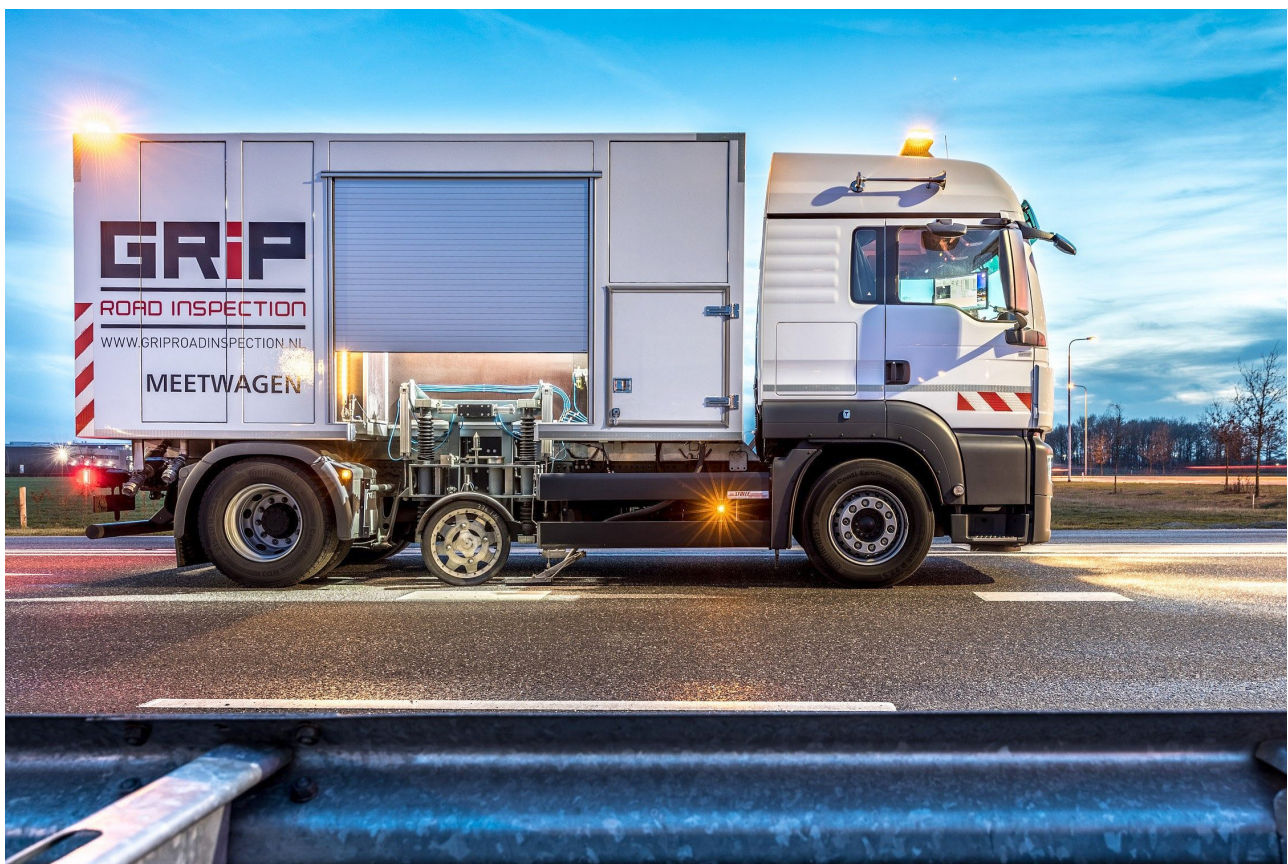
Figure 5: Sideway Force measure truck
